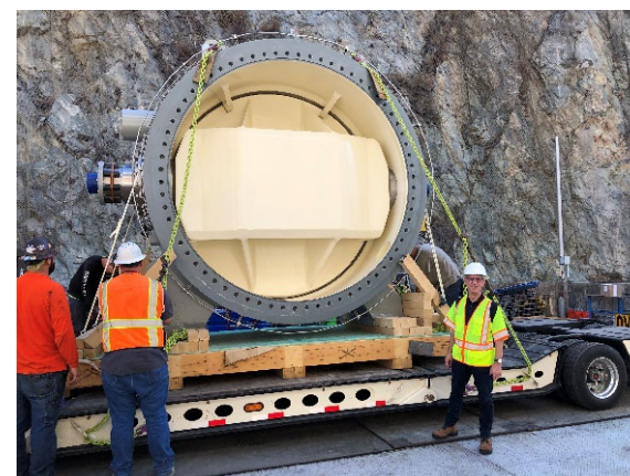
Turbinen Absperrklappe Ø2800mm, 32t, Don Pedro HPP California, U.S.A.
